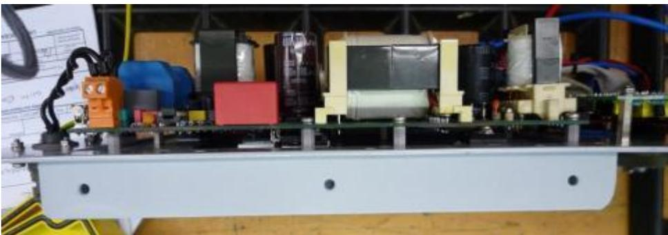
**Pic. 17: Main electronic components on power board on heat sink**
