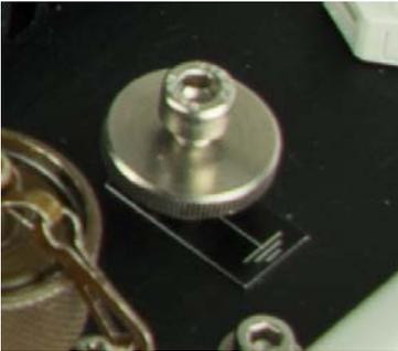
**Pic. 13: Ground connector screw**
